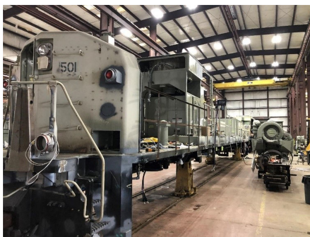
Locomotive in the process of being remanufactured.
